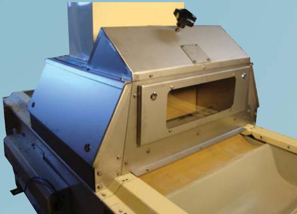
**Simatek Product Dispenser** optimizes the capacity of the bucket elevator. The product dispenser ensures an optimum distribution in the buckets, a gentle product handling, and minimizes product waste. The speed of the elevator can thereby be reduced, and the capacity can be increased.
