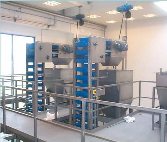
Simatek bucket elevators are available in a closed, dustproof design. When conveying food, open elevators equipped with safety coverings are more common.
