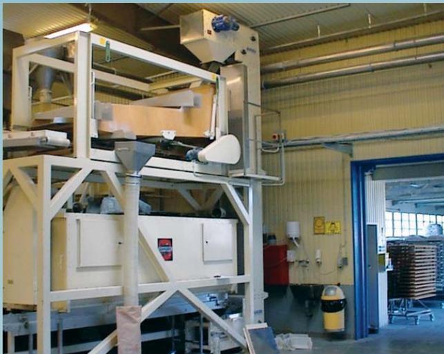
*Elevator construction form C for processing of seed.*
