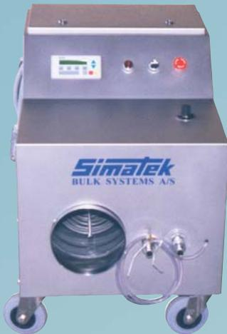
**Simatek Washing Unit** offers facilities for steeping, washing and drying of chains and buckets. One unit can be applied for several elevators.
