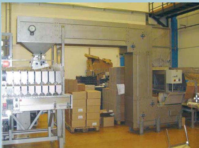
*Simatek bucket elevator construction form A mounted in connection with a weighing system for chocolate and liquorice.*
