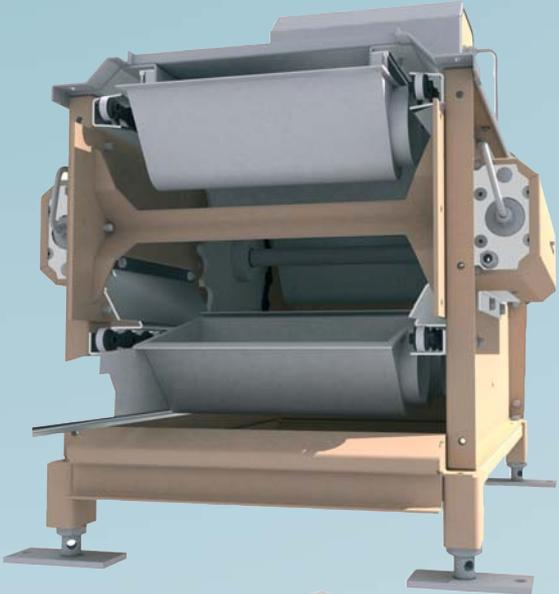
The high-quality chains have been equipped with nylon rollers ensuring long lifetime and quiet operation.
