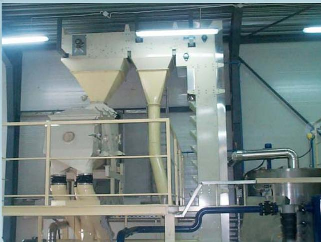
*Elevator construction form C with intermediate outlet. Seed cleaning plant.*
