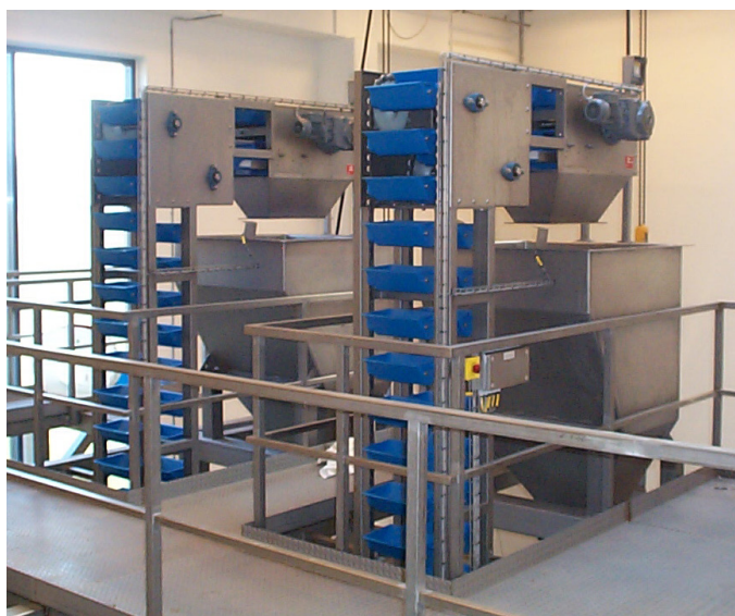
Orkla Confectionery & Snacks Danmark Simatek Universal Elevator conveying snacks
