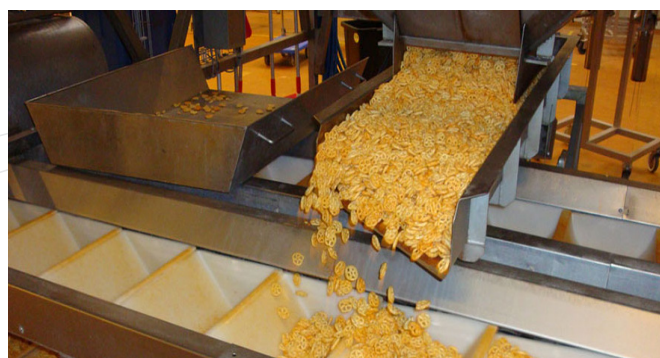
Orkla Confectionery & Snacks Danmark Simatek Universal Elevator conveying snacks
