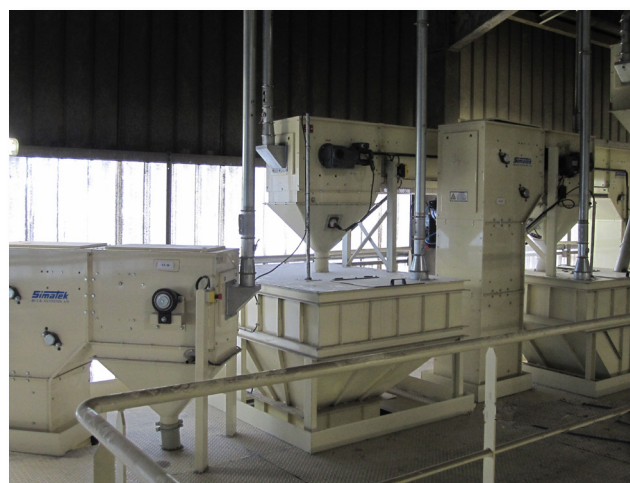
Simatek Universal Elevators conveying various sorts of seeds. Photo: Limagrain, France
