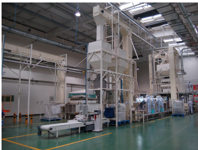
Simatek Universal Elevators conveying sunflower seeds in China. Photo: Sunshine Produce Ltd., China
