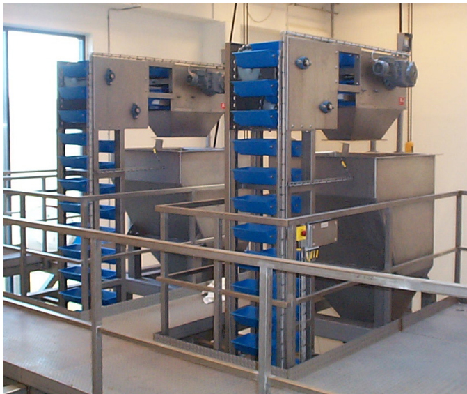
Orkla Confectionery & Snacks Denmark Simatek Universal Elevator conveying snacks
