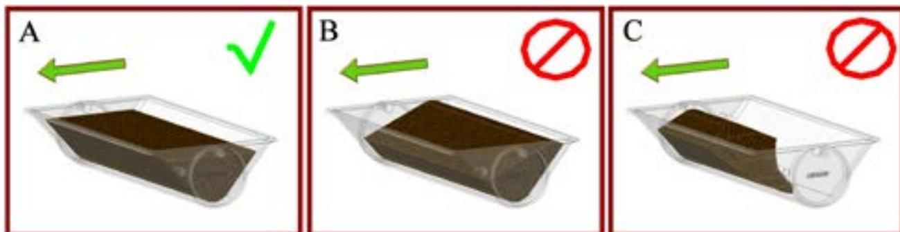
Fig 1. Difference between correct and wrong bucket filling.
